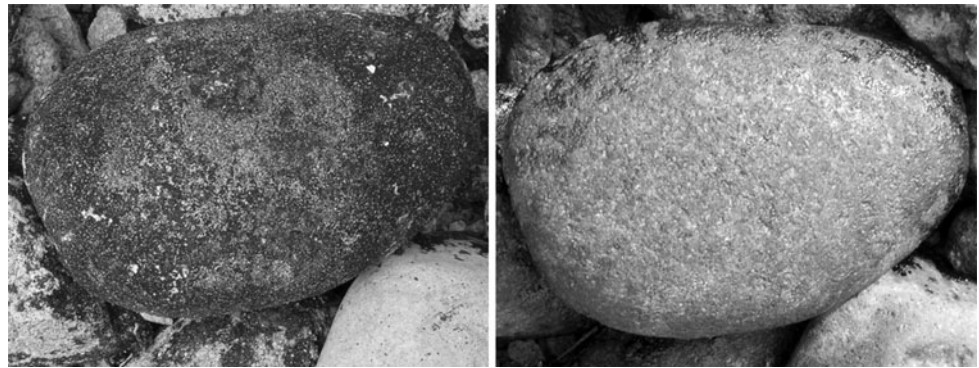
Fig. 6 Detail of a boulder before (left photograph) and after (right photograph) treatment with CytoSol under the conditions specified in the text
