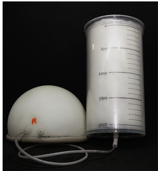
Fig. 1 A picture of the novel device that we used in this study. It consists of a pre-calibrated plastic breast cup which is connected to a reversely calibrated cylindrical jar by a rubber tube
