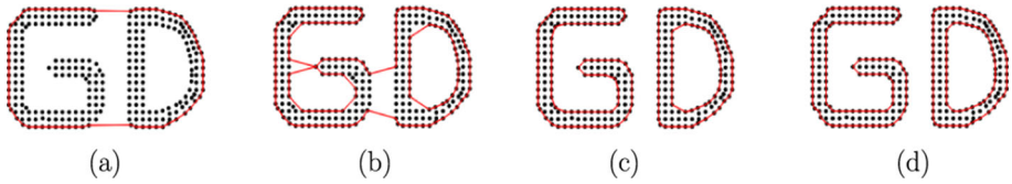
Fig. 7 The \alpha -shapes of P for different values of \alpha . When \alpha = 0 , the \alpha -shape of P is the same as CH(P) . While \alpha increases from 0, the level of details increases in the resultant shape as illustrated in (a)–(d). The values of \alpha in subfigures a, b, c, and d are respectively 0.03, 0.1, 0.2 and 0.9
