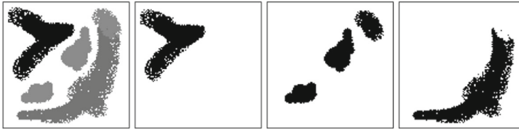
Fig. 1 The discrete data matrix (left) and the three binary matrices derived from it. The binary matrices were created using three discrete values: #0 (left center), #77 (right center) and #237 (right)
