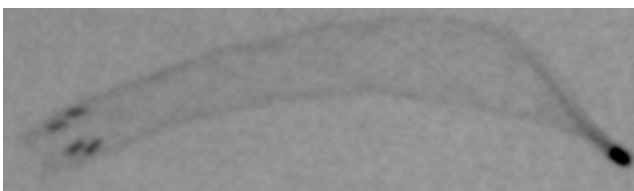
Fig. 2 Fluoroscopy of the prototype FD not implanted in an animal. The five platinum radiopaque markers are clearly visible. The thicker wires measuring 85 \mu m are made of nitinol and the mesh system itself is slightly definable
