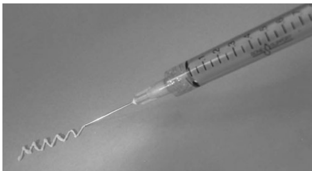
Fig. 2 CERAMENT™ is highly injectable and can be extruded through cannulae with minimum inner diameter of 0.191 cm
