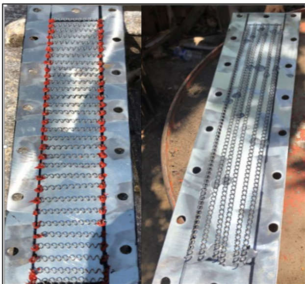
Fig. 4 Production photos of the designed new plate heat exchanger (vertical springs- parallel springs)
