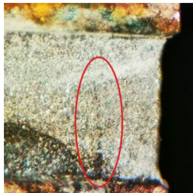
Fig. 4 Microscopic images of thermoelement legs post-thermal cycling, illustrating the presence of a crack in TEG 5 leg (left) and the through-thickness failure of a TEG 6 leg (right)
