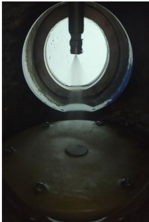
Fig. 8 Droplet distribution of the square nozzle with pore size of 2.4 mm
