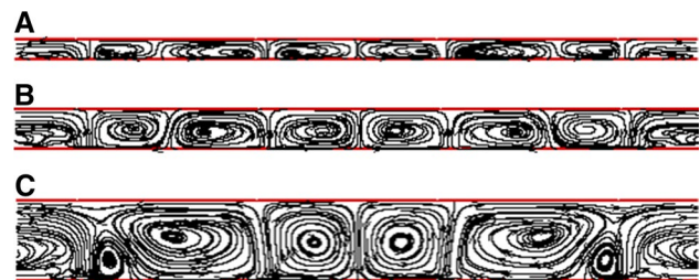
Fig. 5 Computed streamlines images on the mid vertical xy plane for confined jet configuration at S/W = 9 and Re = 10,000 . a H/W = 1 , b H/W = 2 and c H/W = 4
