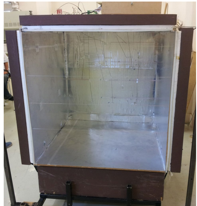
Fig. 2 Experimental cubic open cavity
