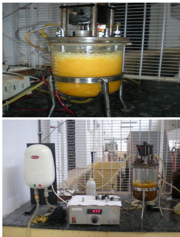
Fig. 1 Laboratory scale biodiesel reactor
