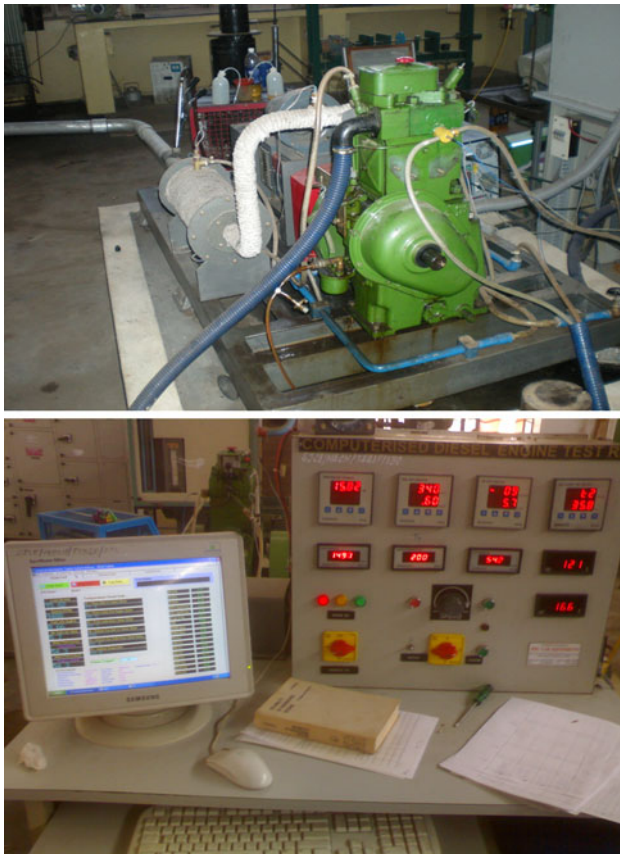
Fig. 2 Computerized CI engine with computer and Display unit
