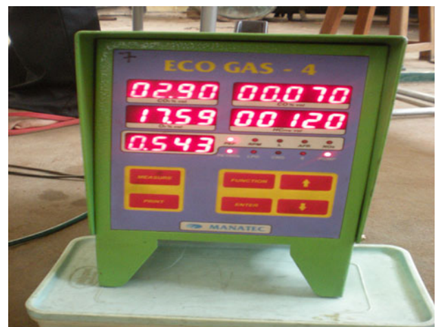
Fig. 3 ECO GAS-4 exhaust gas analyzer
