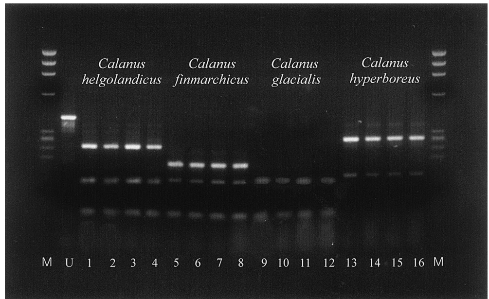
Fig. 3 Calanus spp. Amplification of 16S rDNA from whole adults and subsequent RFLP analysis with restriction endonucleases DdeI and VspI (Lanes 1 to 4, C. helgolandicus ; Lanes 5 to 8, C. finmarchicus ; Lanes 9 to 12, C. glacialis ; Lanes 13 to 16, C. hyperboreus ; M, \phi X174/ HaeIII DNA size-markers; U, amplified uncut C. helgolandicus DNA)
