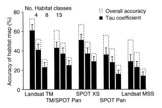
Fig. 2 Comparison of satellite sensors for mapping coral-reef habitats of Caicos Bank, showing overall accuracies and tau coefficients (error bars upper 95% confidence intervals of tau coefficient). Three levels of descriptive resolution are described for each sensor: coarse (4 habitat classes), intermediate (8 habitat classes) and fine (13 habitat classes). (See Tables 1 and 2 for explanation of sensor abbreviations and definition of habitat classes, respectively)
