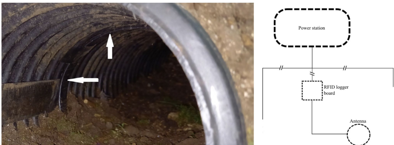
Fig. 2 Automatic passive integrated transponder (PIT) tag detector installed in a rhinoceros auklet artificial burrow. The antenna (white arrows) is placed inside the tunnel so that individuals entering or exit-
