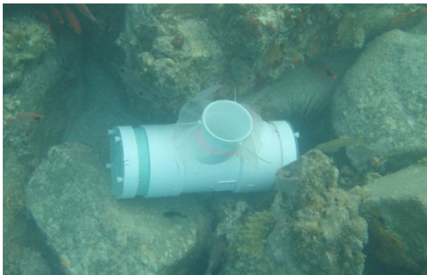
Fig. 2 Photograph of submerged trap (visual plus olfactory)
