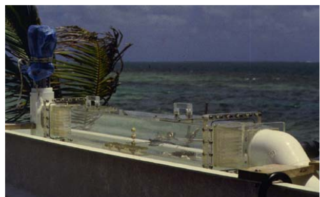
Fig. 2 Photograph of flume/respirometer inside the temperature-controlled reservoir. The working section is UV-transparent acrylic and is 11 \times 10 \times 110 cm in dimension. Algal turf-covered plates sit in a depression in the floor of the flume and a hot-film thermistor flow probe is located 0.8 cm above the plates
