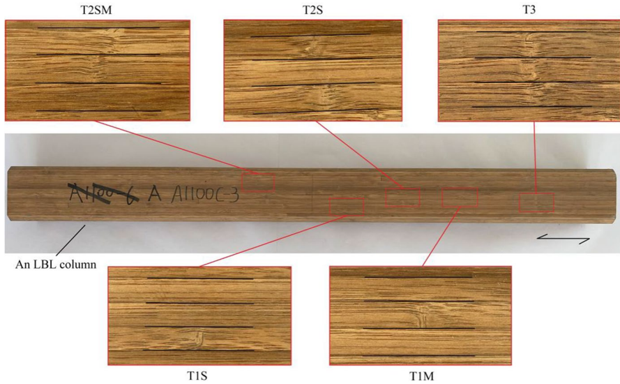
Fig. 2 Node distribution of an LBL column
