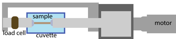
Fig. 6 In the tensile stage, the sample is fixed in between two clamps and fully immersed in solution. Main components of the setup are: a load cell (in bold on the left) to control and measure axial tensile forces, and a linear motor (on the right) to control and measure the strain
