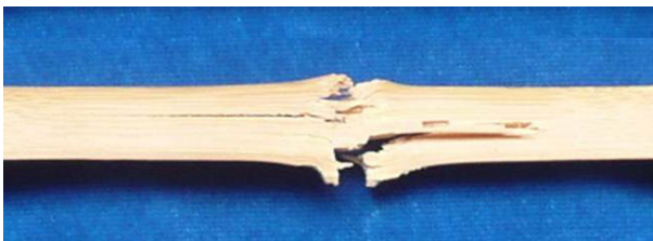
Fig. 7 Photograph (taken from Shao et al. 2010: figure 4) showing part of a tensile test specimen containing a node. After application of tensile force, cracking has started in the nodal region and is spreading longitudinally. Reproduced with permission from the Forest Research Institute, Malaysia
