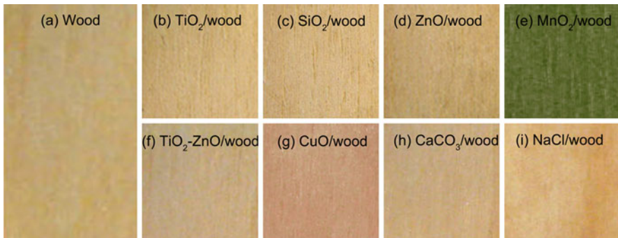
Fig. 3 Macroscopic images of a unmodified wood and b–i different nanomaterials/wood ( b TiO 2 , c SiO 2 , d ZnO nanorod arrays, e MnO 2 , f TiO 2 –ZnO, g CuO, h CaCO 3 , i NaCl)
