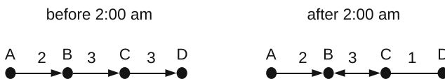
Fig. 3 Illustration of permanent loops with widest path routing in a linear 4-node network: the widest path successors toward destination D are demonstrated with arrows and the numbers above links show available link bandwidth in Gbit/s at the given time
