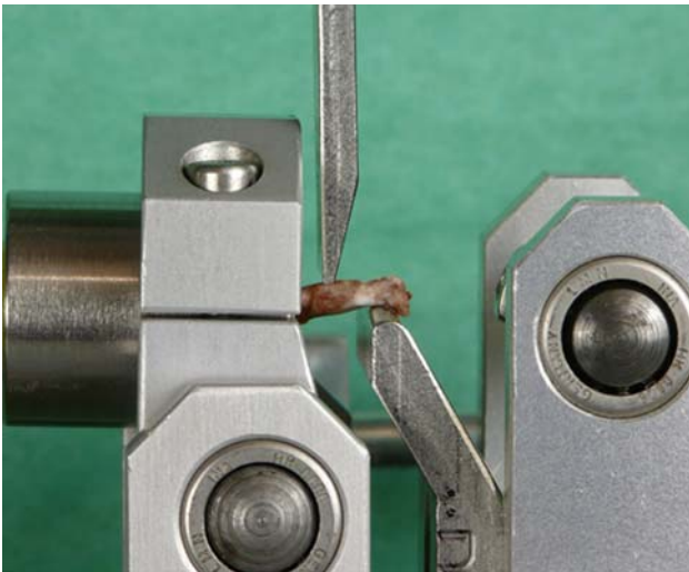
Fig. 2 Three-point bending test of a mouse femur
