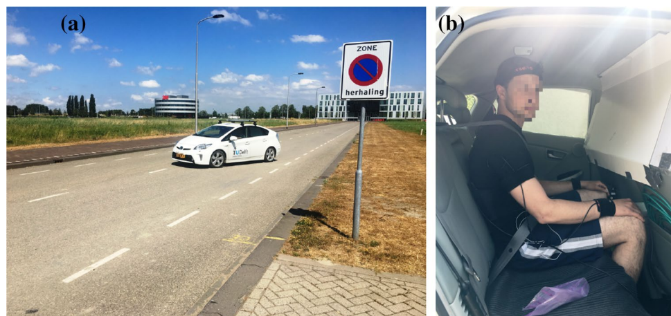
Fig. 1 Experimental setup. Left is the Prius 2013 model on the test road used during the experiments in the process of performing a slalom. Right shows the internal vision condition where the external view to the sides and front is blocked
