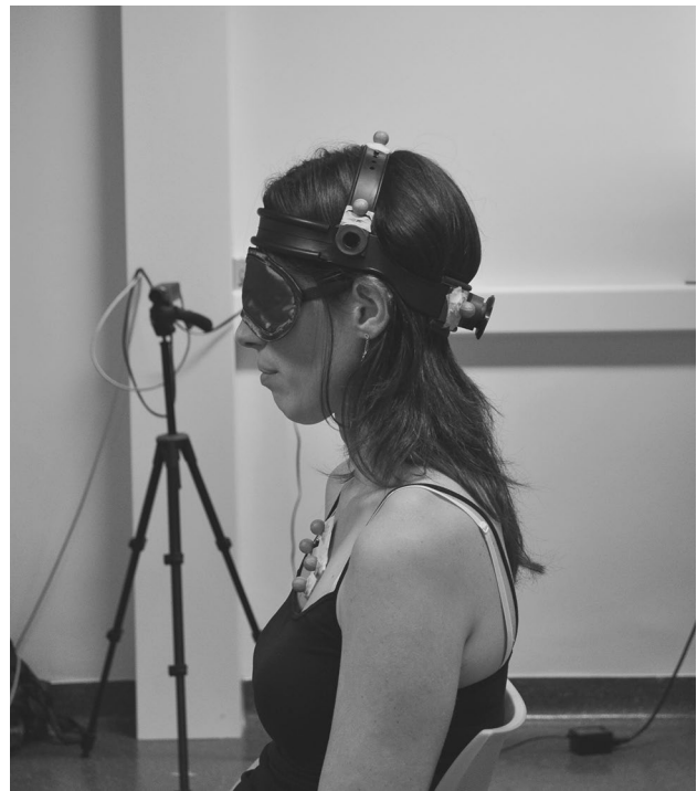
Fig. 2 Sensor placement of VICON ® system for the head repositioning accuracy task
