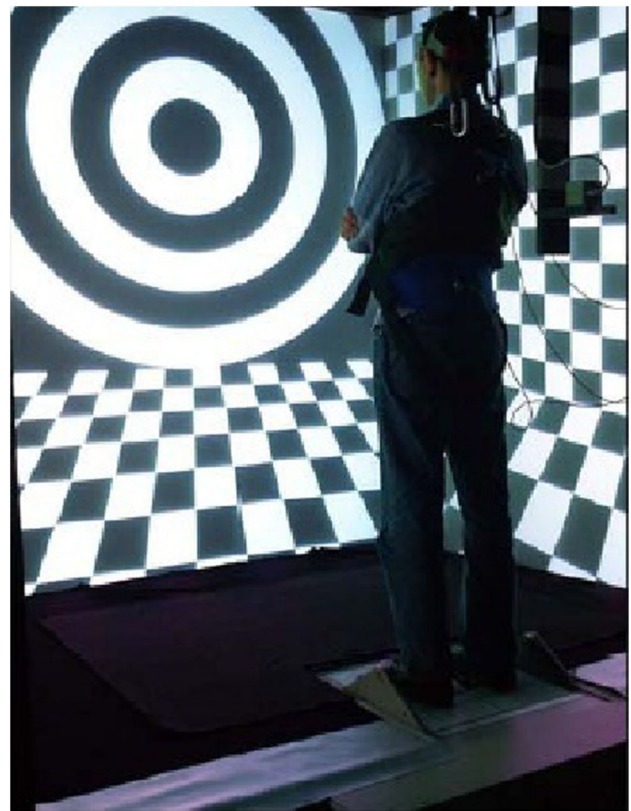
Fig. 2 Experimental setup for second balance test with participant standing in the BNAVE and visual stimulus projected onto screens
