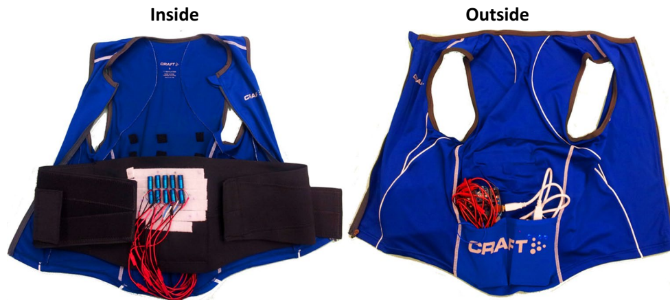
Fig. 1 Vibrotactile vest used in experiments 1 and 2. Motors are attached to a back brace to ensure that they are pressed firmly against a participant's back. The controller and battery pack reside in pockets on the back of the vest. The motor layout shown is used in experiment 2
