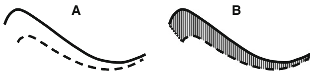
Fig. 3 Method involved in determining the area enclosed between two curves. Solid curve is the actual footpath, while the dashed curve is the desired footpath. See the section of “ Data processing ” for the details of calculating this area
