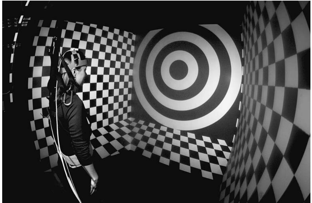
Fig. 1 Schematic of experimental set-up. Subjects stood upright on force platform that was able to pitch up and down in proportion to body sway. The optic flow environment consisted of alternating black and white squares on the side walls ( > 30^\circ from midline) and alternating black and white concentric rings on the front wall
