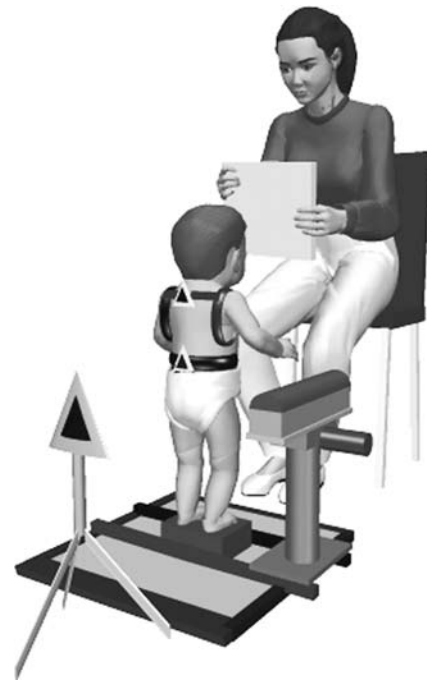
Fig. 1 An infant standing on the small pedestal in a hands free condition. To the right is the instrumented touch apparatus. Behind the infant is the Logitech receiver and the small triangles on the infant's torso are transmitters for the six-dimensional position tracking system. The caregiver and second experimenter are excluded for simplicity of presentation
