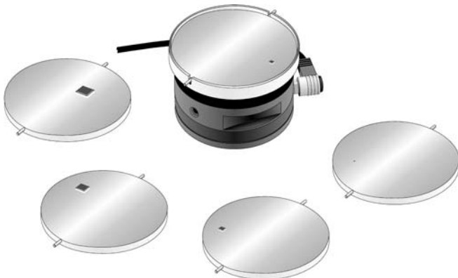
Fig. 1 The ATI six-axes force and torque sensor with the receptacle holding a 1.0-mm raised square target. Disk diameter: 7.5 cm. The size and position of the four other raised targets are shown below. The recessed squares are not shown
