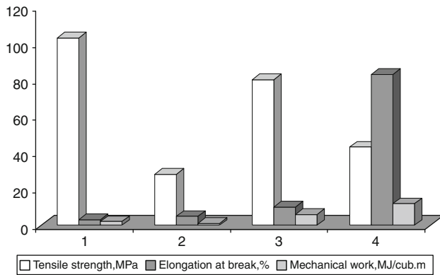
Fig. 7 Mechanical properties of chitosan films containing different amounts of plasticizer: 1 0%; 2 5%; 3 10%; 4 20%
