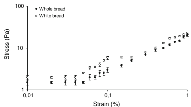
Fig. 2 Strain dependence of stress profiles for commercial pan bread samples (frequency 1 Hz)
