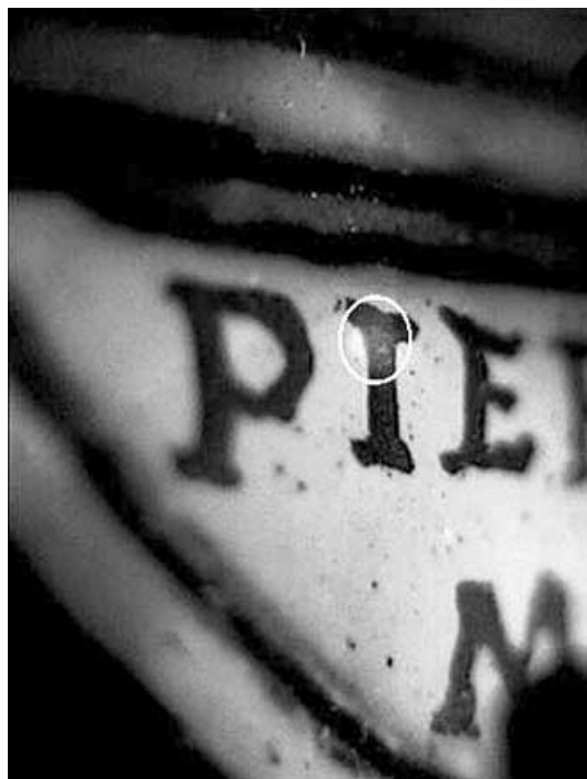
Fig. 9 Detail of an artist's signature on a 16th c. Limoges painted enamel (line thickness app. 150 \mu m). The ellipse represents the area lit by the overlaid red positioning diode spots
