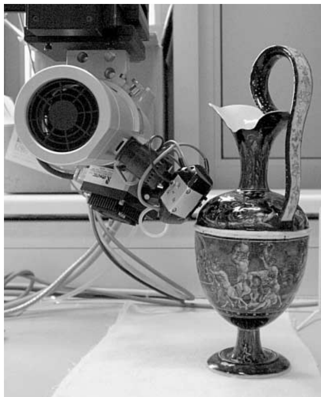
Fig. 10 \mu -XRF investigation of a Limoges painted enamel (jug dated "1564" with bacchus procession) in the Kunstgewerbemuseum Berlin
