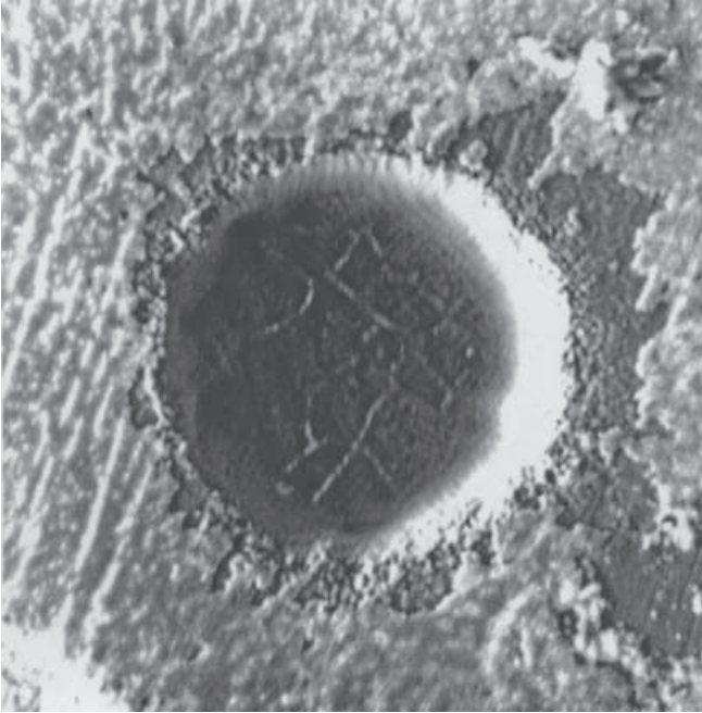
Fig.4 SEM photograph of a 100 µm ablation crater in SRM NIST 610 (100 pulses at 70 mJ/pulse laser output)
