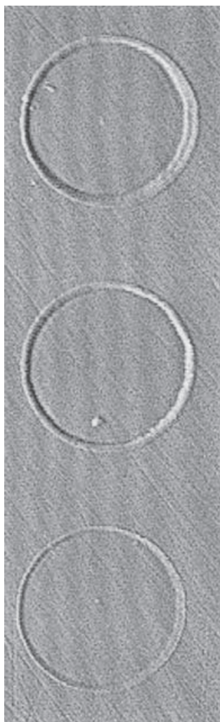
Fig. 13 SEM picture after 1, 2 and 3 pulses per crater onto aluminium oxide (60 nm removal per shot) to determine degree of destruction of a gemstone sample
