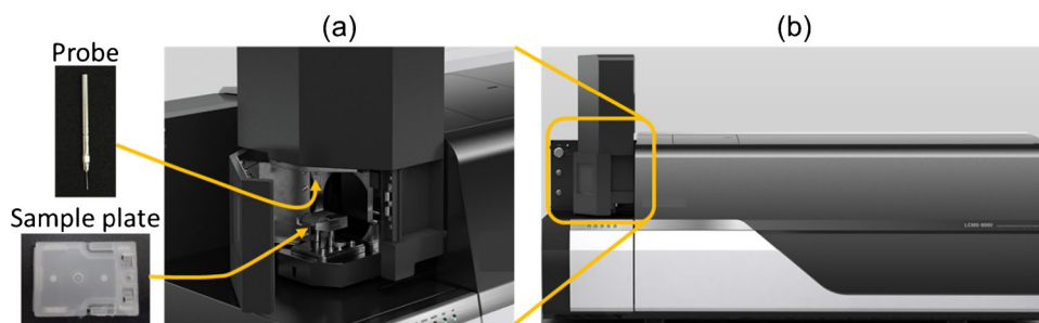
Fig. 1 Photographs of the a detail of the PESI ion source and b exterior of the PESI-MS/MS
