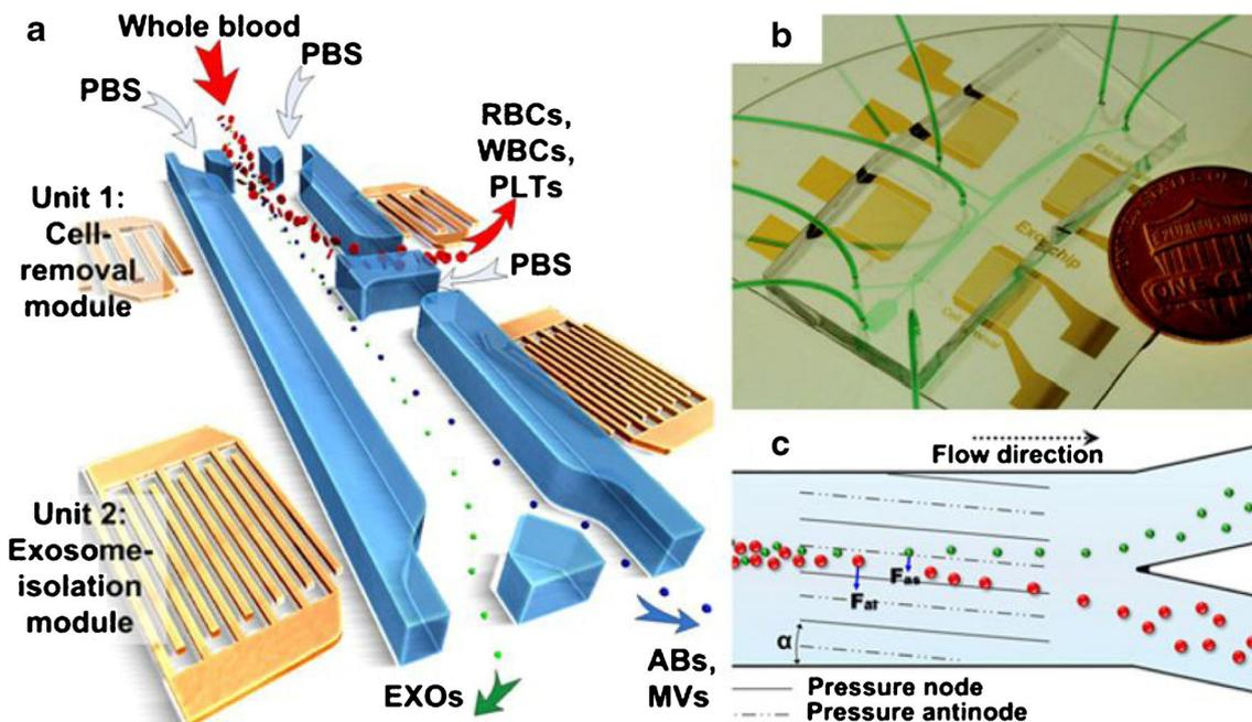
**Fig. 4** Schematic illustration of and mechanisms underlying the integrated acoustofluidic device for isolating exosomes [58]. **a** Red blood cells (RBCs), white blood cells (WBCs), and platelets (PLTs) are filtered by the cell-removal module, and then subgroups of exosomes [apoptotic bodies (ABs), exosomes (EXOs), and microvesicles (MVVs)]
