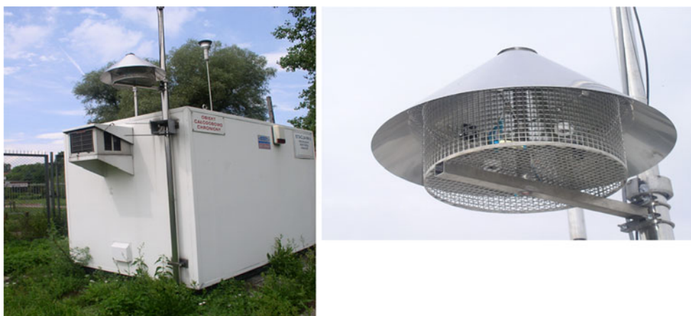
Fig. 2 Radiello passive samplers were placed in a specially designed stainless shelter during the exposure period at the monitoring station
