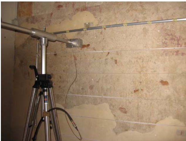
Fig. 3 Unilateral NMR instrument while measuring the moisture content of the northern wall in San Rocco church
