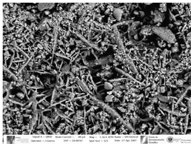
Fig. 7 SEM-BSE image of the surface of a typical black crust of lenticular gypsum crystals (with dust particles trapped in the network) on the patina SPU-29. Scale bar 10 \mu\text{m}
