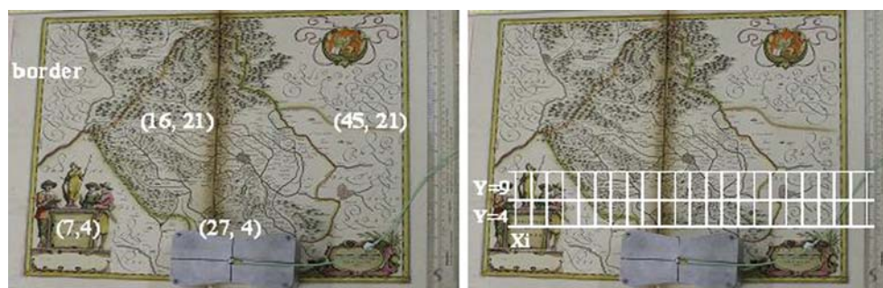
Fig. 1 Left: points on the map at which T_1 relaxation times were measured. Right: points on the map at which T_2 relaxation times were measured. The probe head used for the measurements is also shown
