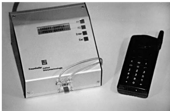
Fig. 8 Photo of an eight-channel potentiostat with flow cell and DNA-chip in front
