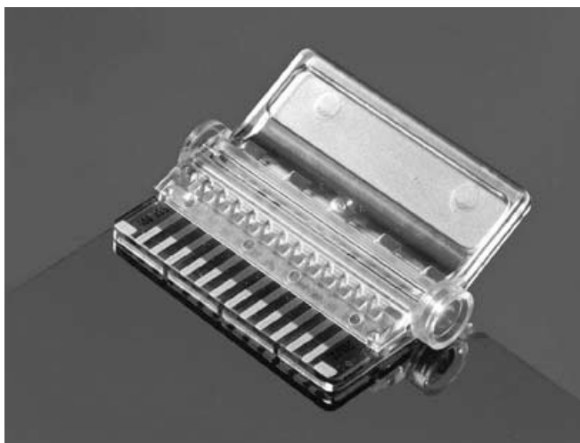
Fig. 4 Picture of the fully assembled Roche thick film biosensor cassette, ready to use
