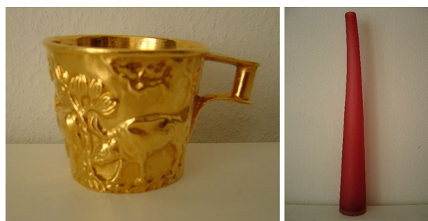
Fig. 1 The color of metallic gold and gold nanoparticles in ruby glass. Reprinted from ref. Corain et al. (2008) with permission from Elsevier Science
