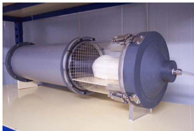
Picture 2 Continuous flow through whole body inhalation cages. Rats were individually housed for individual telemetry purpose. Cages were made of PVC and polycarbonate to be suitable for telemetry signal recordings. Reception antenna are placed under the rat housing volume for most efficient telemetry signal recording
