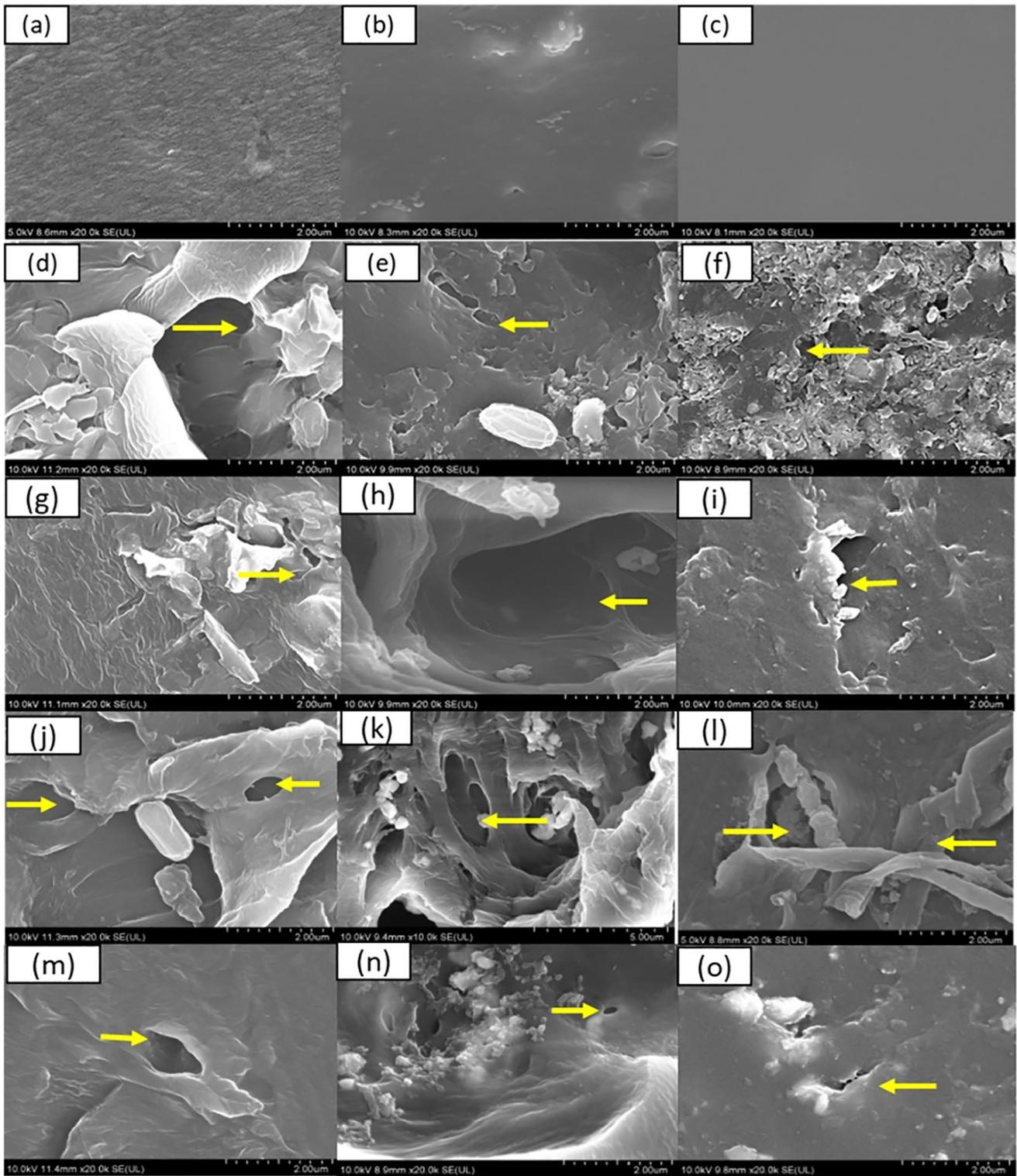
**Fig. 8** FESEM micrographs showing the surface appearance of (a) control LDPE; b control PET; c control PS; d MR5-treated LDPE; e MR5-treated PET; f MR5-treated PS; g MR10-treated LDPE; h MR10-treated PET; i MR10-treated PS; j BS5-treated LDPE; k BS5-
