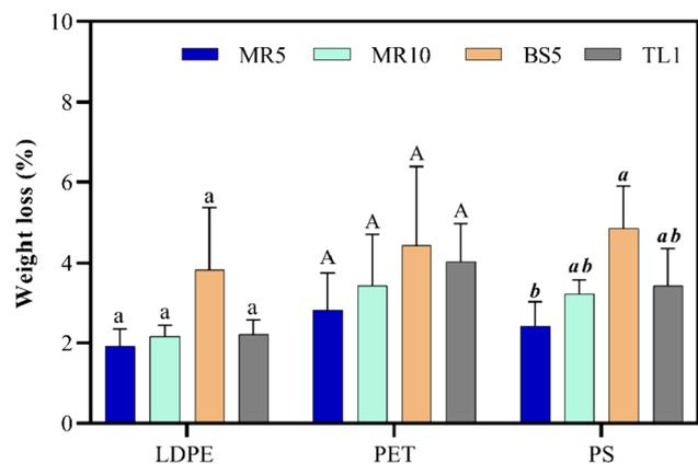
**Fig. 7** Measurement of weight loss of the LDPE, PET, and PS with bacterial isolates MR5, MR10, BS5, and TL1 after 4 weeks of degradation. Error bars indicate the standard error ( $n=3$ ). Values followed by the different letters are significantly different within sampling days
