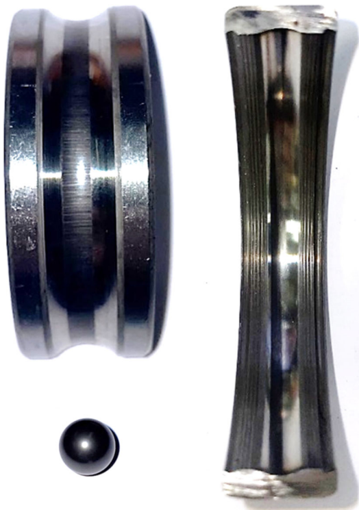
Fig. 5 DE bearing at 500 r/min and 10 A
