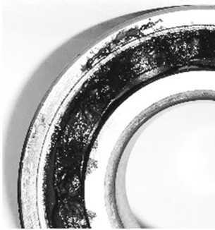
Fig. 3 Lubricant darkening due to discharges
