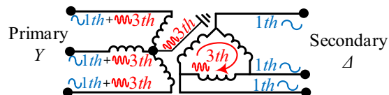
Fig. 5 Transformer connection for eliminating the 3th-harmonic component
