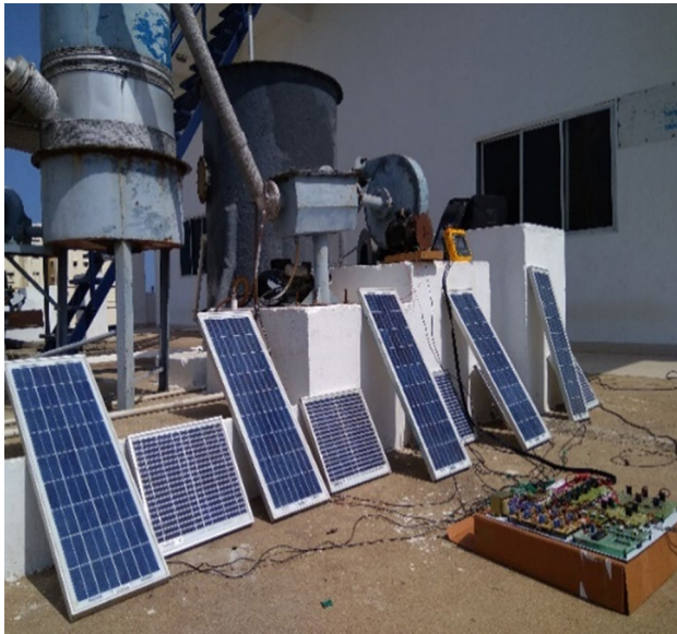
Fig. 18 Experimental setup of PV panels with MMI
