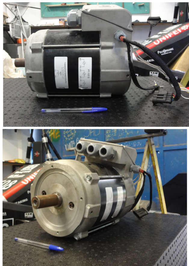
Fig. 1 Induction motor (IM) structure. A machine used in the electric propulsion system of Formula SAE light electric vehicles
